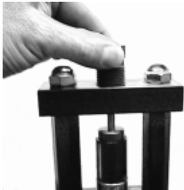
The die screws into the head of the press, replacing the floating punch holder in Corbin swaging presses. It has a 7/8 X 14 thread for types -R, -M, or -S, or 1-1/2 X 12 for type -H. The punch fits into the press ram. In type -R die sets, the punch fits the shell holder slot of the reloading press (without a shell holder present). In type -M and -H sets, the punch screws directly into the press ram like a swaging die.
